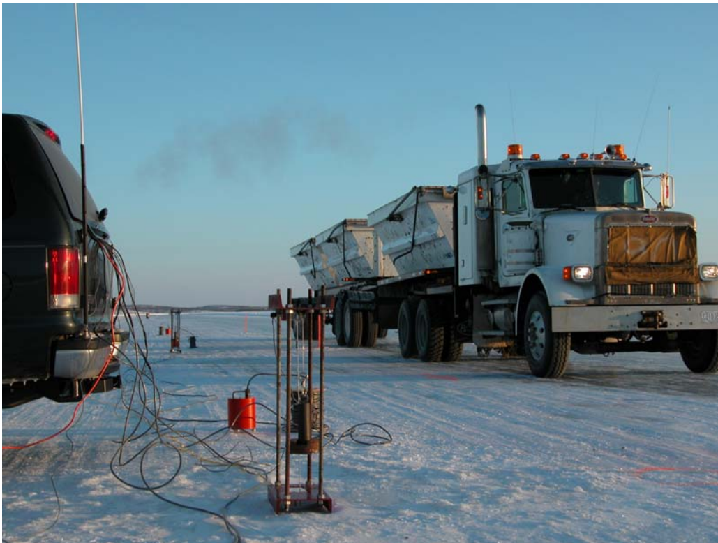
FIGURE 11 Ice Deflection Field Trials.
