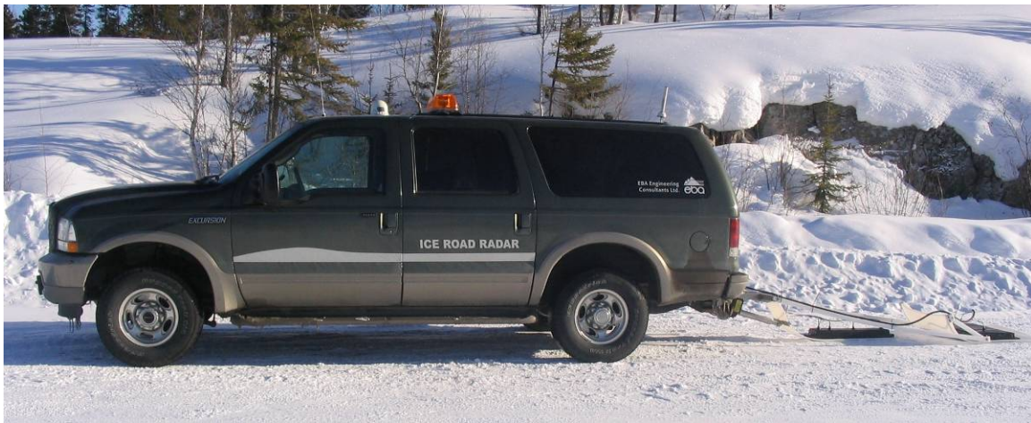
FIGURE 6 ICE ROAD RADAR™ System Survey Vehicle.
