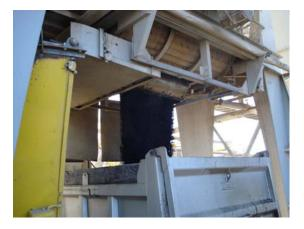
Figure 3 – Loading WMA Into Truck Box
