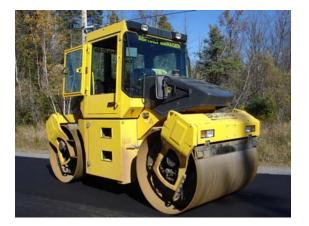
Figure 4 – Vibratory Roller on WMA Section
