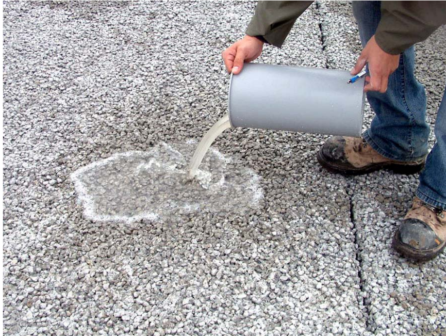
Figure 4. Visual Assessment of Permeability (Trial Slab)
