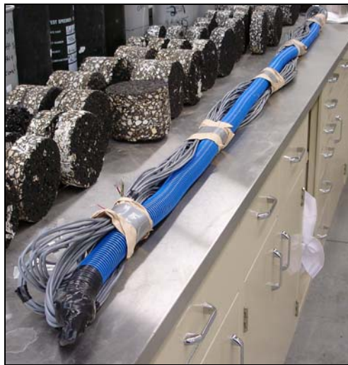
Figure 17. Thermistor assembly prior to installation.
