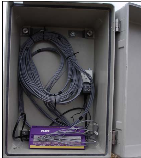
Figure 20. An example of the instrument enclosure with DT800, power source and telephone access.
