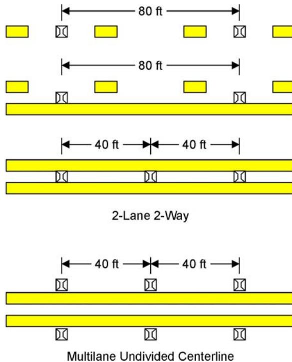
**Figure 2. Recommended Layout of Raised Pavement Markers (RPM)**
