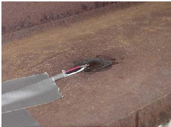
**Figure 13. Strain Gauge Mounted on Girder**
