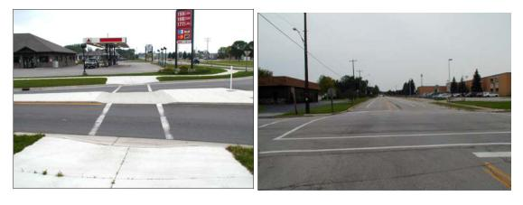
Figure 6.2 Pedestrian crossing accommodations at the Lineville/Cardinal Roundabout compared (left) to a regular intersection (right) (Brown County, WI)
