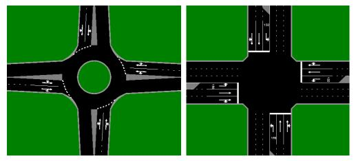
Figure 7.3 Intersection layouts—roundabout (left); signalized intersection (right) (aaSIDRA)
