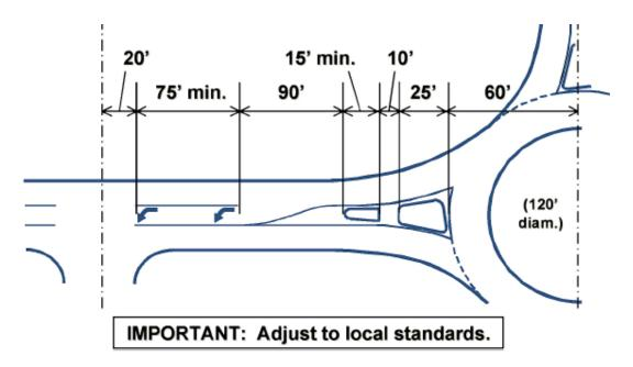
Figure 5.3 Left turn access near a roundabout (KSDOT, 2003)
