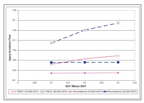
Figure 3.23 Predicted crashes for roundabouts versus two-way stop control (Robinson et al, 2000)
