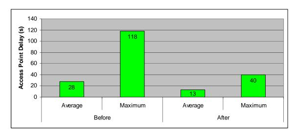
Figure 5.4 South Golden Road access point delay before and after roundabout installation
