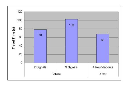
Figure 3.8 South Golden Road travel times before and after roundabout installation
