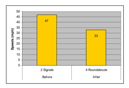
Figure 3.9 South Golden Road 85th percentile speeds before and after roundabout installation
