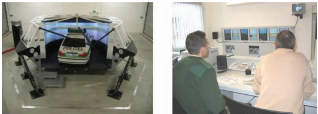
Figure 1 The driving simulator with motion platform and projection system (left) and observation facilities (right)
