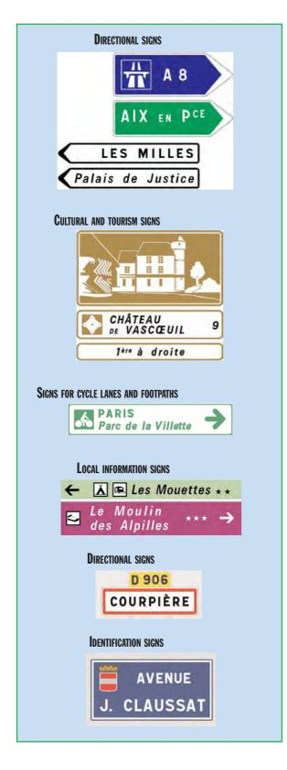
This helps give users information from their point of departure to their point of arrival. These are necessary for carrying out their journeys in optimum conditions of comfort and safety. For road signs to be efficient it is necessary to:
