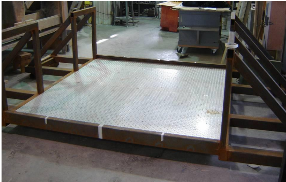
Figure 20: Physical Model of the Stainless Steel/Aluminum Panel
