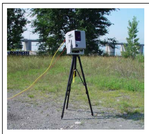
Figure 2 – Scanneur CYRAX 2500 (Cyra Technologies Inc.)
