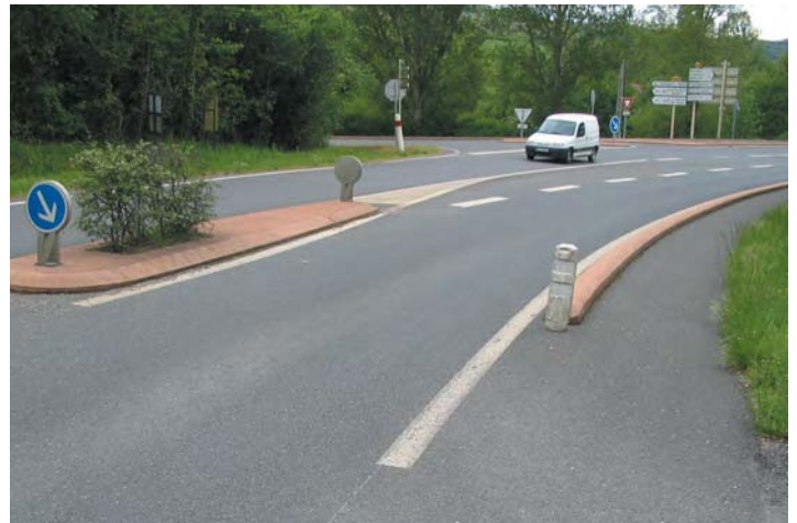
Bypass : the cyclist is protected behind the separator (FFCT S. Jackson)
