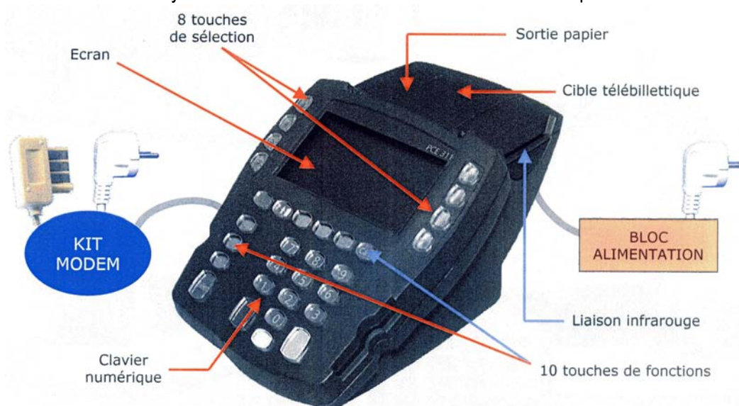
Figure 7 : Le terminal Point de vente Service commercial – source : Sytral
