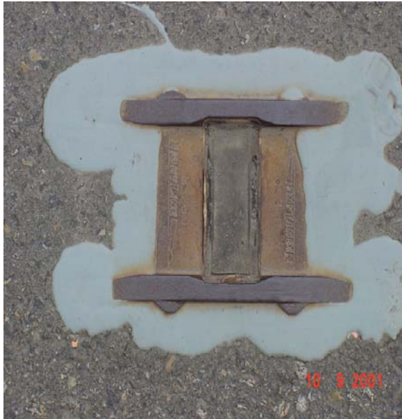
3M reflective marker dislodged from nightline shoe
