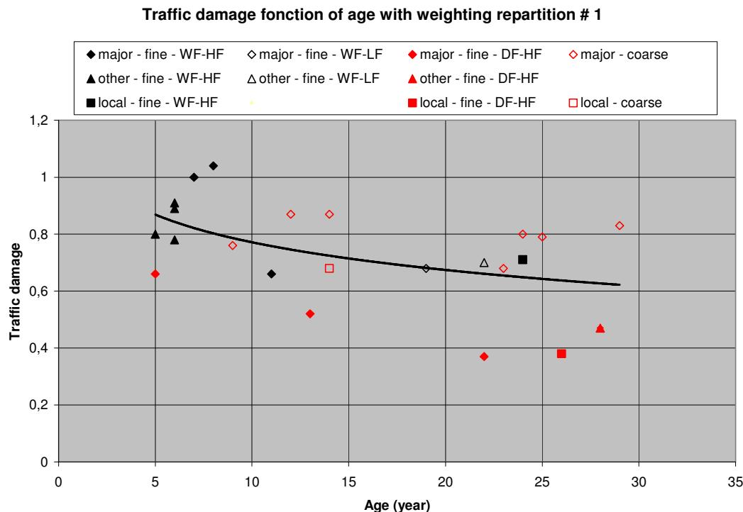
**Figure 4-2: Relationship between damage ratios and pavement age (for weights distribution 1)**
