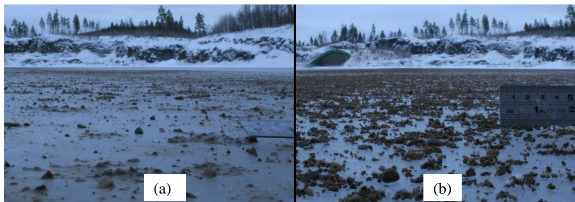
Figure 12. (a) Applied sand (150 g/m 2 ), pre-wetted with 30 vol% hot water on an iced surface. (b) The same type and amount of sand applied without the water.
