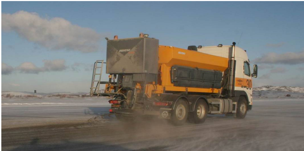
Figure 2. Sand spreader with warm, pre-wetting functionality.
