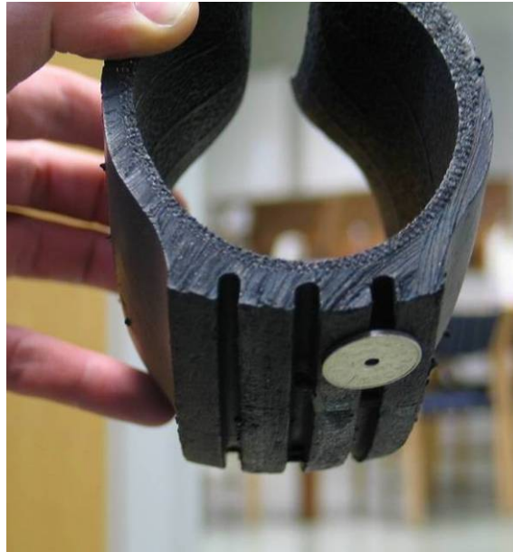
Figure 22. A coin pressed against the sticky measurement tire stayed adhered while hanging upside down.
