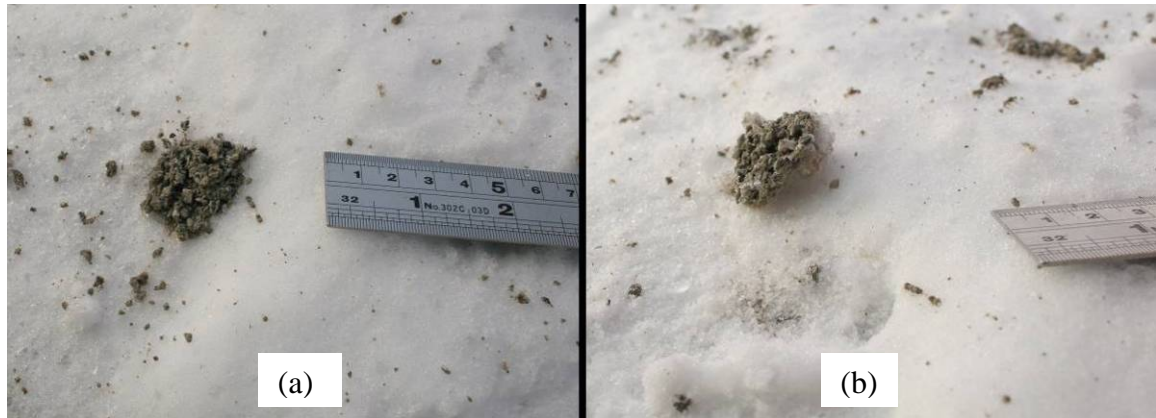
Figure 10. (a) Lump applied on loosely bonded snow. (b) Rubbing caused the lump to break loose in one piece.
