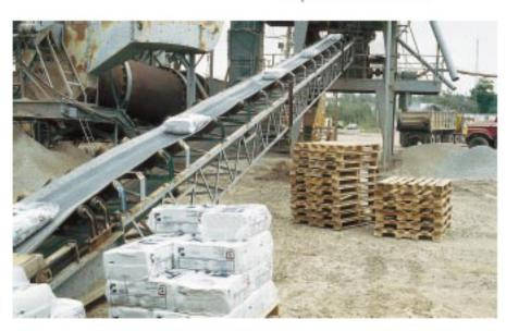
Adding asbestos fiber into the pugmill at the asphalt batch mix plant.
