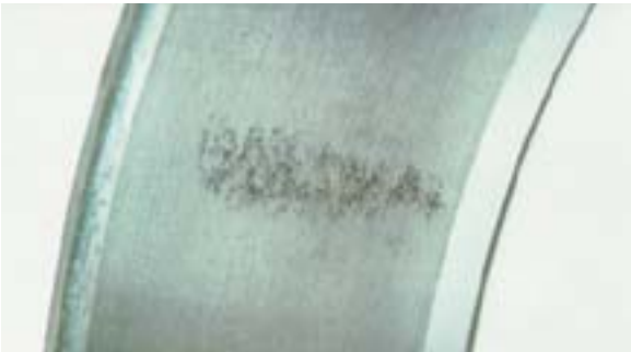
Figure 2 Pieces of metal or grit in the lubricant.
