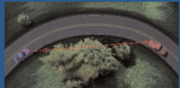
Lsd in horizontal curve situation
