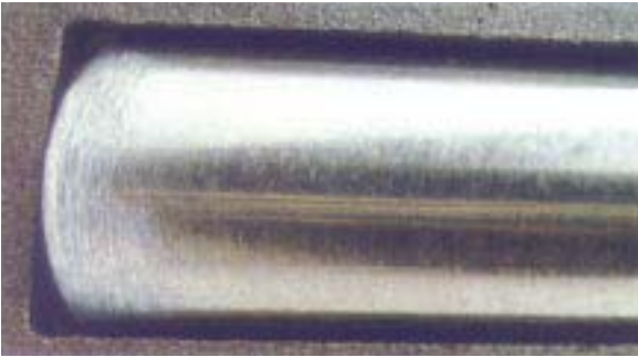
Figure 4 Chipping on the outer edge at the widest diameter of the tapered roller: indicates that bearing is too tight .
